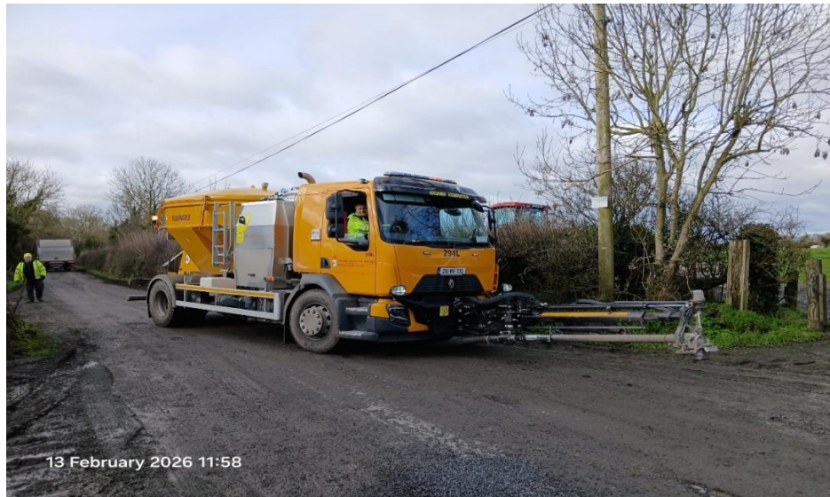
New Velocity Patcher (Pothole repair machine) February 2026
