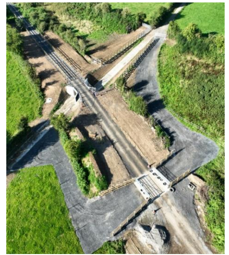
Various images along Lot 5A – showing public lighting plus grade-separated and at-grade agricultural crossings
