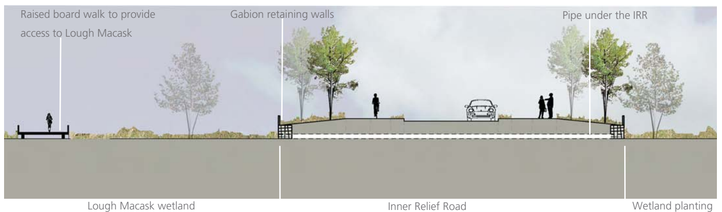
Fig. 36. Section H - Inner Relief Road, and Lough Macask
