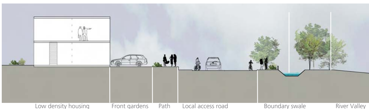
Fig. 34. Section F - Southern Boundary of the LAP Area (adjacent to the Bregagh River Valley), through swale
